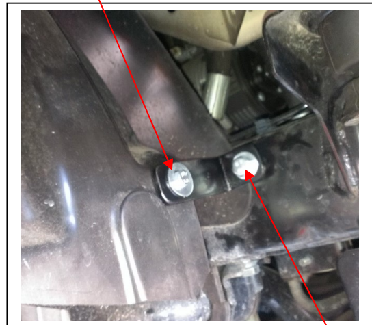
Figure 10 M8 x 1.25 x 25 bolt, flat and spring washer into captive nut
