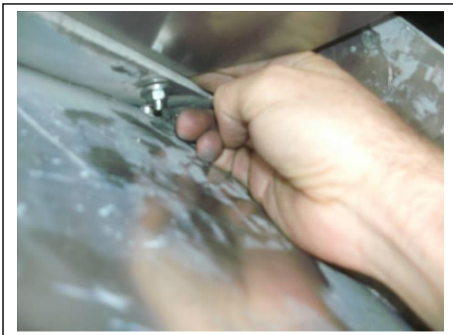
Figure 29: Placing bolt in from side of under body guard.
