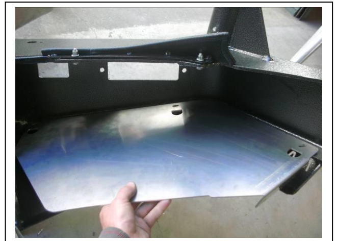
Figure 28: Placement of under body guard. Bumper removed for photo.
