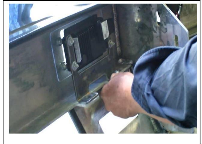
Figure 20: Attach mount to lower leg of channel
