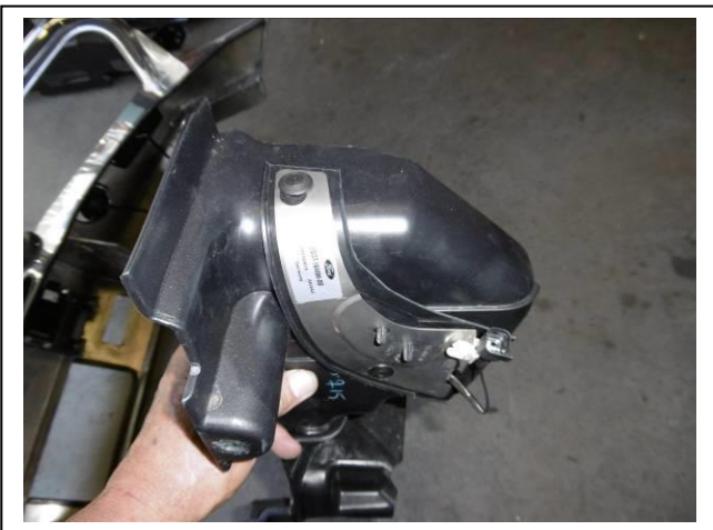
Figure 9: Bend aerial carefully to the shape of the dam and drill in the holes already in place
