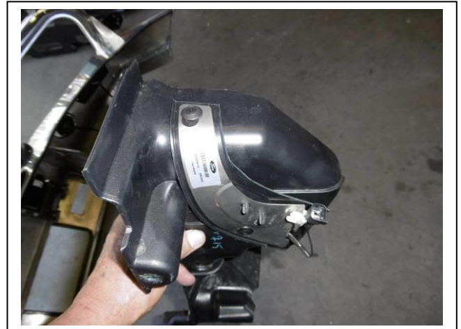
Figure 9: Bend aerial carefully to the shape of the dam and drill in the holes already in place
