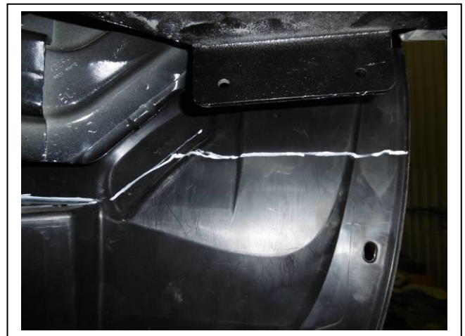
Figure 30: Using underbelly guard as a guide trim wheel
