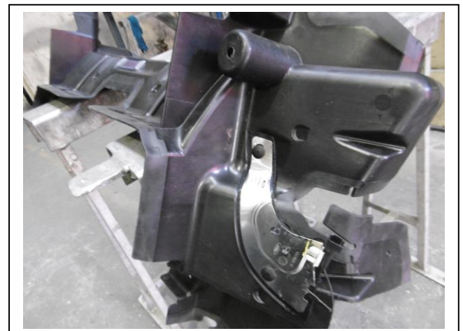
Figure 10a EVEREST: Bend aerial carefully to the shape of the dam and drill in the holes already in place
