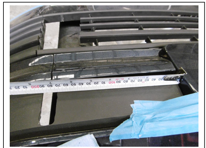
Figure 8: Lower blanking grille cut. NOTE: Take measurement from mount supplied with Protection bar
