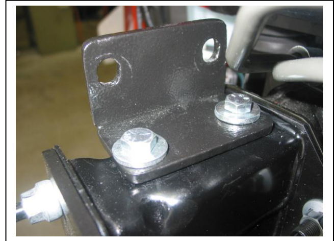
Figure 8: Top mount support – drop bolts in from top
