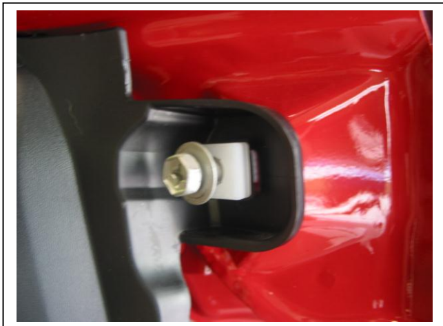
Figure 3: Re insert plastic clip from headlight section into front of flare.
