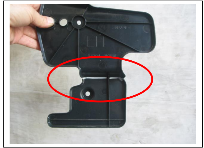
Figure 2: Trim lower section from air dam. Passengers side shown.
