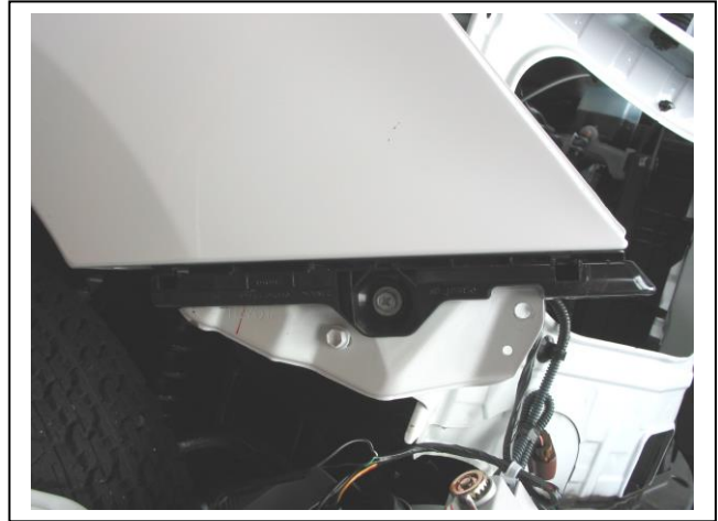
Figure 6 - Remove plastic bumper support from under guard.
