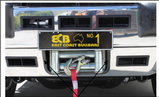
Attach 6mm clip lock
