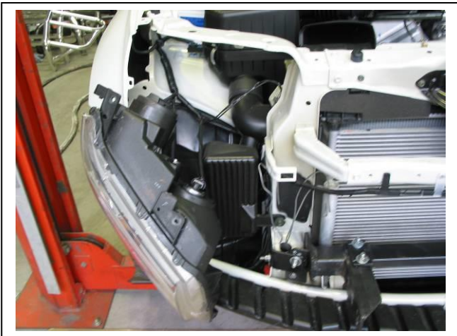
Figure 7 – Drivers side shown Headlight assembly moved forward to access wiring
