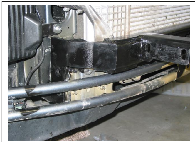
Figure 3 – Placing steel mounting bracket, ready for installation, Turbo diesel vehicle.
