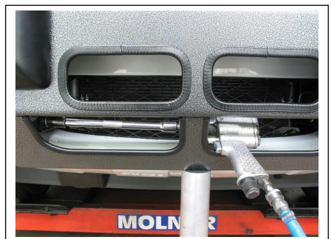
Figure 16 Impact wrench access for nuts
