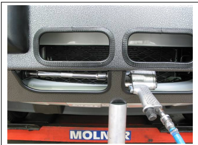
Figure 15 Impact wrench access for nuts
