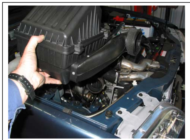
Figure 1 – Removing air cleaner housing
