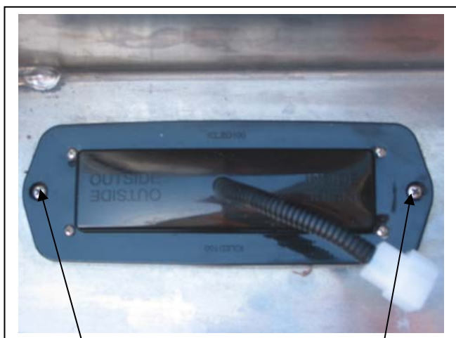
Figure 7 Stainless steel self-tappers
