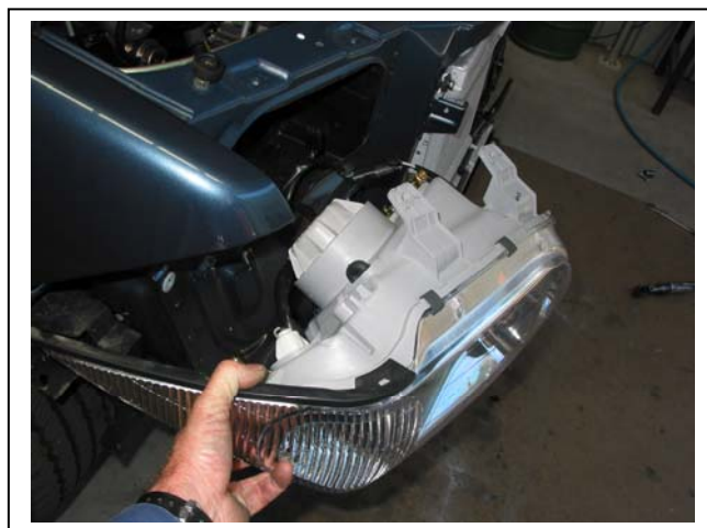
Figure 2 – Moving headlight forward to access wiring
