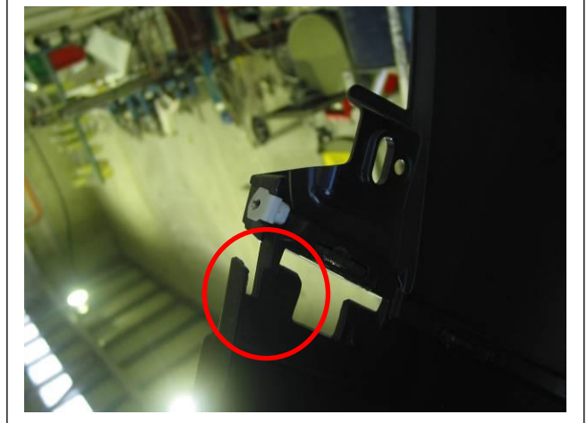
Figure 8 – Plastic clip reused to secure inner guard to flare.
