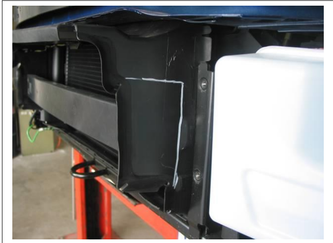
Figure 7 – Passenger side shown. Remove section including air dam brace.
