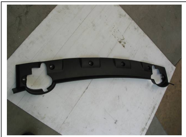
Figure 11 – Trim driver's side to match original passenger side cut out
