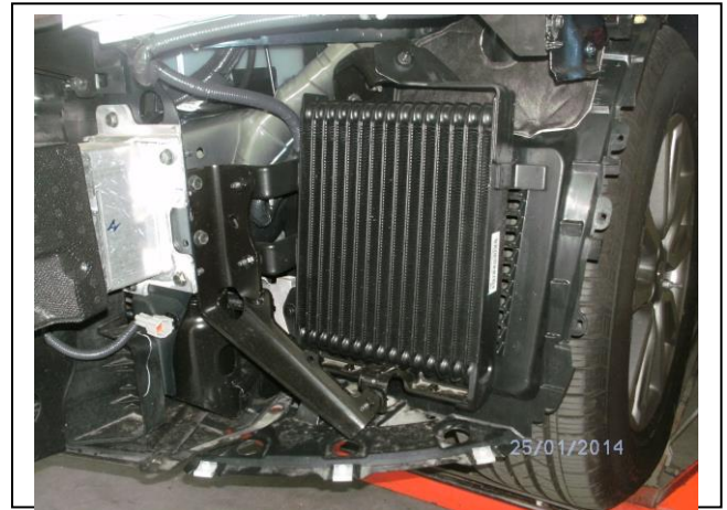
Figure 4: Recommended fog light disconnection point, passengers side.
