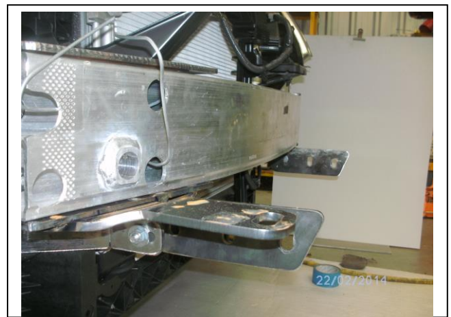
Figure 8: bumper support and mount fitted to vehicle.
