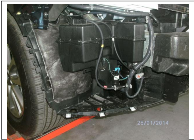
Figure 3: Recommended fog light disconnection point, drivers side.
