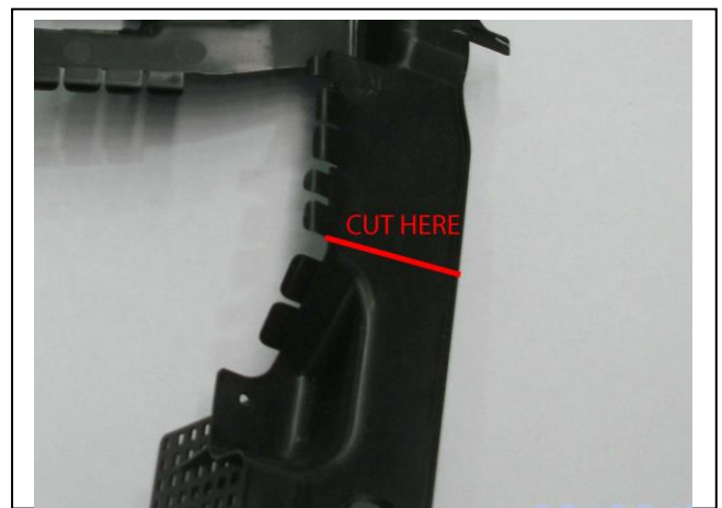
Figure 6: Cut line for passengers side air dam
