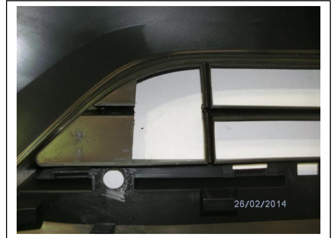
Figure 10: Bumper cut to allow mount protrusion
