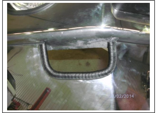
Figure 16: Clip lock trim in tow point opening
