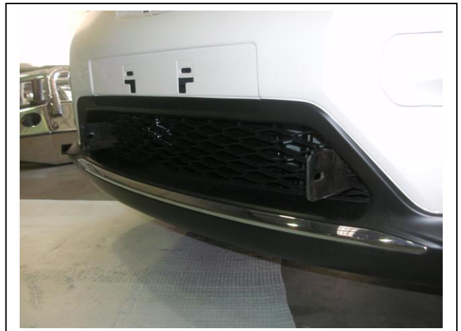
Figure 12: ECB steel Mount with bumper fitted
