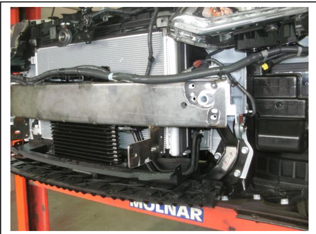
Figure 5: ECB Steel mount fitted.
