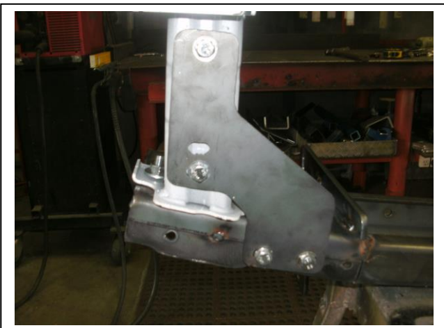
Figure 7: Top mount gusset, removed from vehicle for photo
