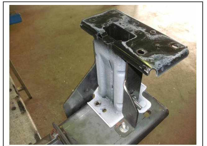
Figure 8: Lower mount gusset, removed from vehicle for photo
