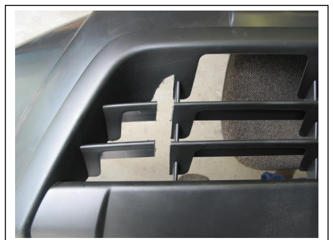
Figure 4: Trim grille to measurement of mounts.
