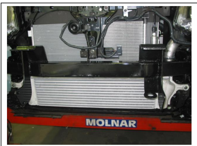
Figure 3: ECB mount bracket installed
