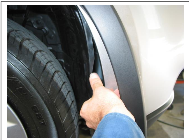
Figure 1: View of Flare, removed from guard
