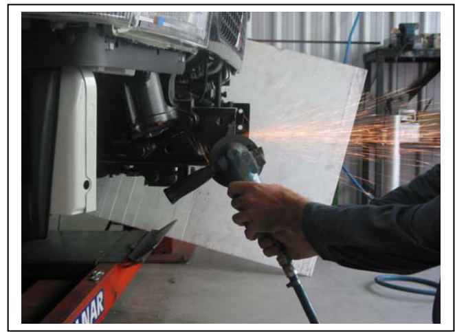
Figure 2 – Grind off remaining weld. Drivers side shown
