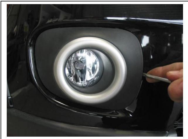
Figure 7: Use a flat bladed screw driver to carefully remove fog light covers.
