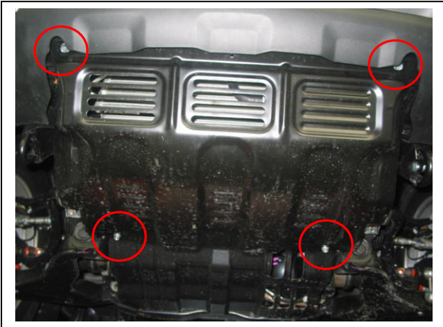
Figure 1: Under body guard bolts to remove.
