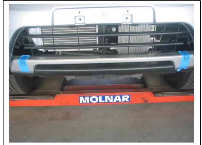
Figure 2: Grille trim to accept steel mount.
