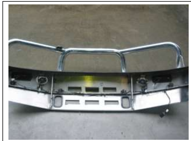
Figure 13: wiring harness wired into rear of Protection bar
