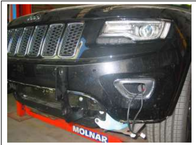
Figure 3: Bumper with lower section fully removed.
