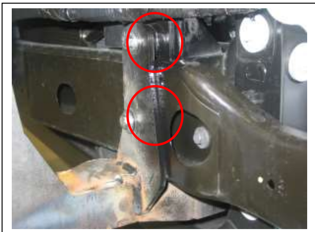
Figure 5: ECB steel mounting brackets showing spacer placement
