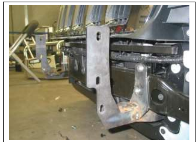
Figure 6: ECB steel mounting brackets fitted. Bumper removed for photo.
