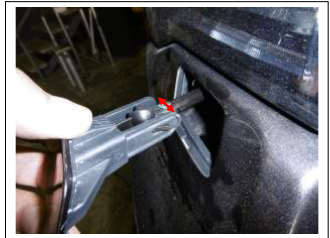
Figure 4: Removal of washer covers. Pull edges to sides.
