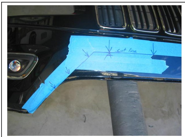
Figure 13: side tape line on bumper. NOTE: Cut line on tape is to the inside.
