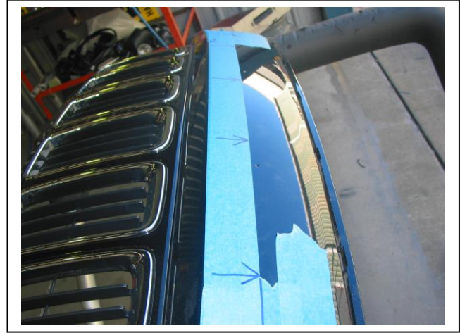
Figure 12: Top tape line on bumper. NOTE: Cut line is to bottom of tape.
