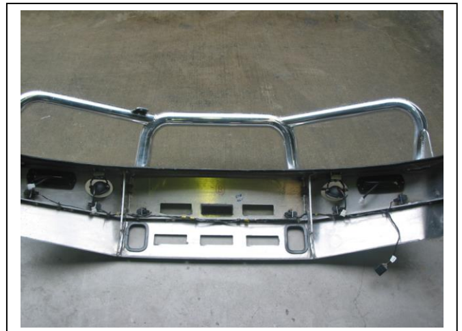
Figure 20: wiring harness wired into rear of Protection bar
