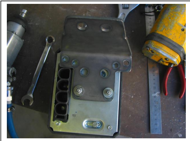
Figure 9: Warn control box with ECB control box mount fitted
