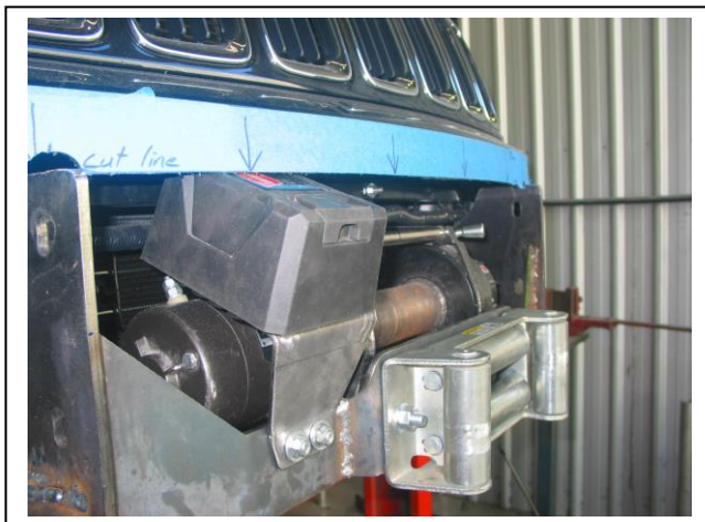
Figure 11: Warn control box mounted to winch frame.
