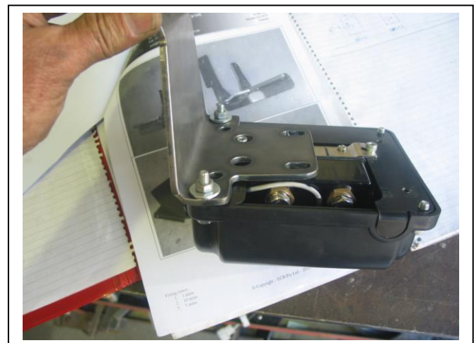
Figure 8: Mean mother control box with ECB control box mount fitted
