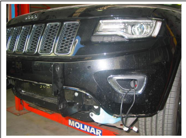
Figure 3: Bumper with lower section fully removed.
