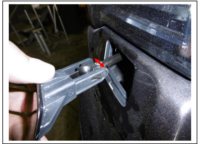
Figure 4: Removal of washer covers. Pull edges to sides.
