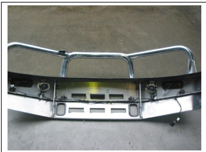
Figure 11: wiring harness wired into rear of Protection bar
