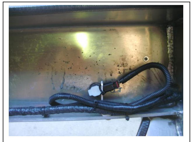
Figure 12: Parking sensor finish mounted.
