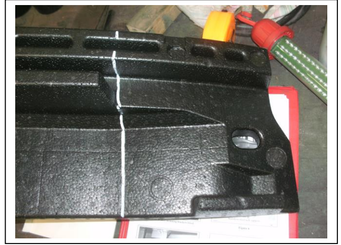
Figure 4: Trim ends off polystyrene bumper support too allow access for ECB steel mounts.
