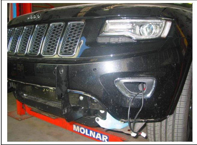
Figure 3: Bumper with lower section fully removed.
