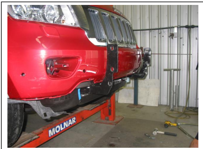
Figure 5: ECB steel mounting brackets fitted. With bumper fitted.
