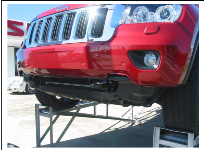
Figure 3: Bumper with lower section fully removed.
