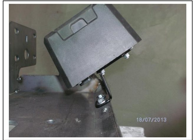
Figure 8: Warn winch control box mounted. Winch removed for photo.
