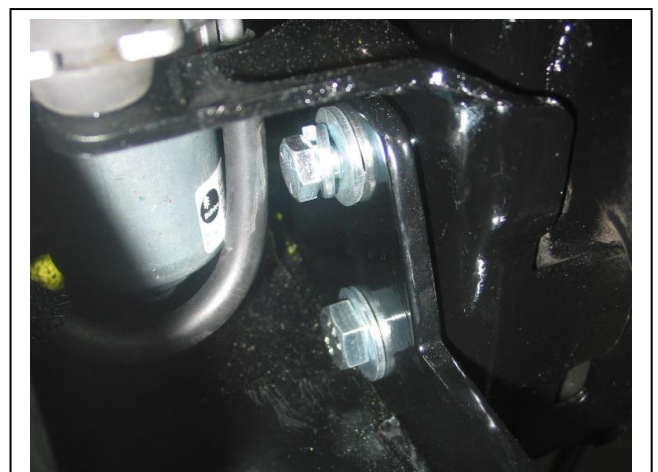
Figure 12: Access point for rear bolts
