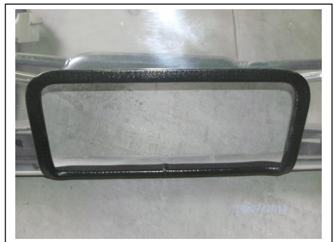
Figure 18: winch opening trimmed. Note joint to bottom.
