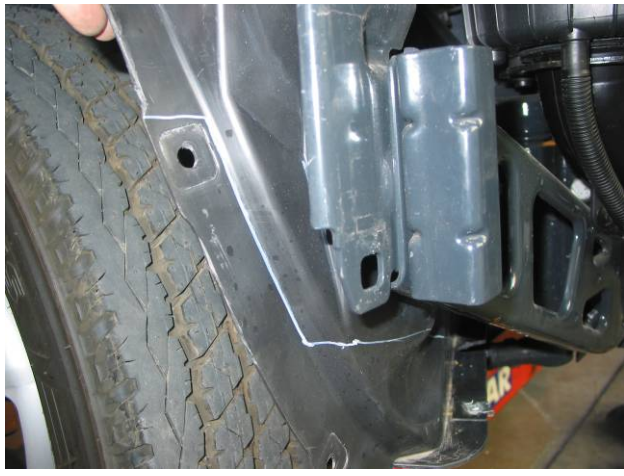
Figure 4: Marking inner guard for trim using bumper support as guide
