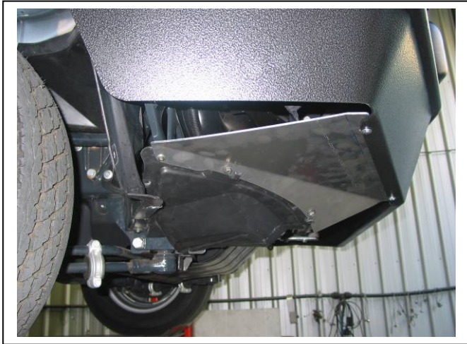
Figure 10: Underbody guard fitted, Drivers side shown
