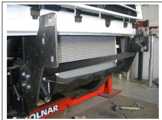
Figure 3: ECB Steel mounting system fitted
