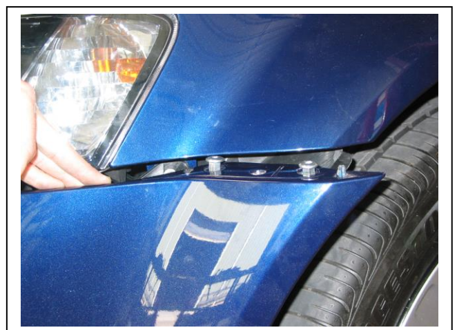
Figure 12 – Passenger side shown. Loosely fit original nuts and bolts to make it easier to refit bumper cover.
