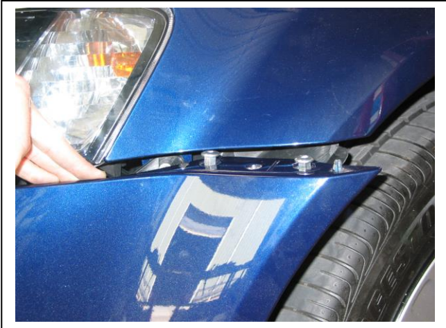
Figure 13 – Passenger side shown. Loosely fit original nuts and bolts to make it easier to refit bumper cover.
