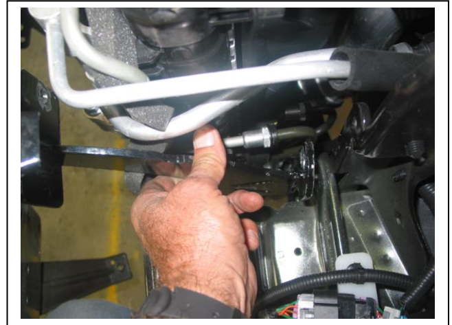
Figure 2: Slide ECB crash can support between chassis mounting and radiator support.
