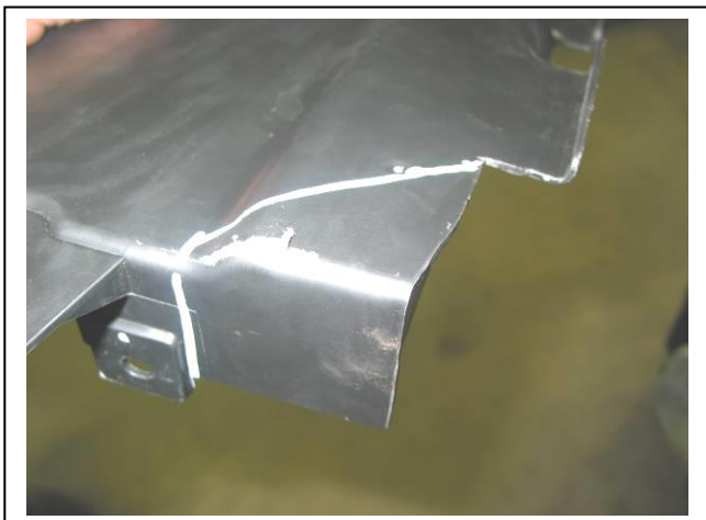
Figure 5: Bottom corner of drivers side air dam. Trim along white line.
