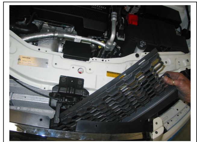
Figure 12: Slide trimmed grille behind bumper and clip into place.
