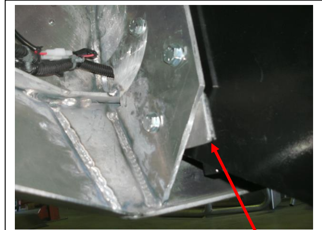
Figure 12 – 2 spacers used to adjust Protection bar to centre. This body was off centre by 5mm.
