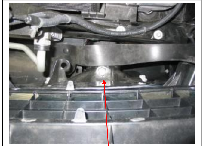
Figure 2: 21mm bolt looking down from behind grille
