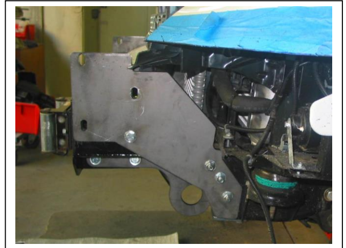
Figure 6: Mounting of winch frame to chassis mount
