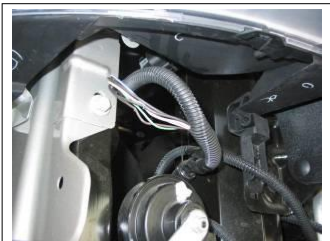
Figure 7: Wiring harness under driver's headlamp
