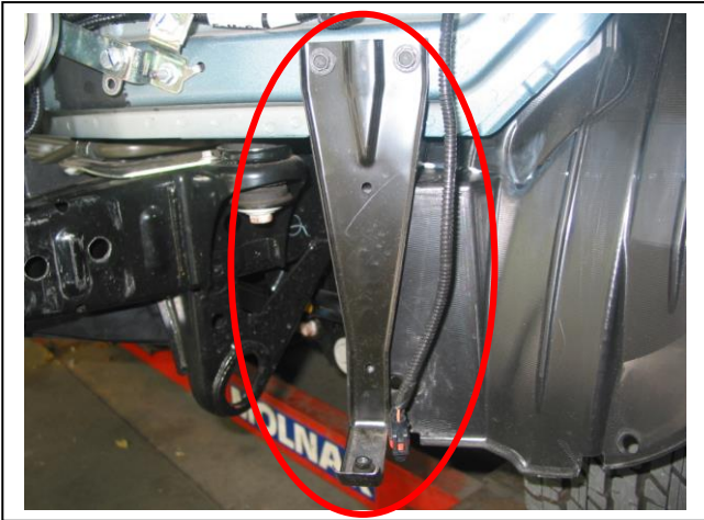
Figure 8: Remove side lower bumper supports. Use removed bolts to fit ECB inner guard supports
