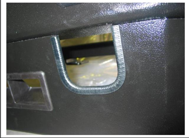
**Figure 10:** 3mm clip lock trim fitted
