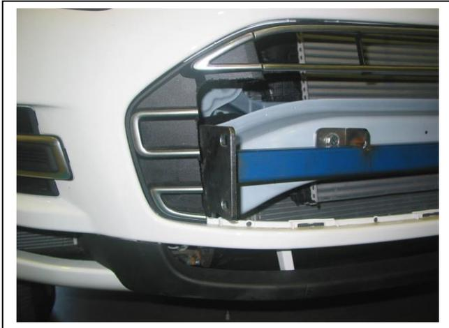
Figure 5: Grille fitted to vehicle.
