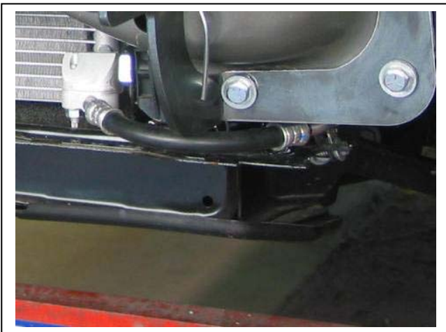
Figure 3: Check clearance between ECB steel mount and air conditioning pipe
