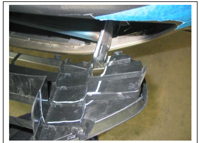
Figure 4: Align and mark grille for trim
