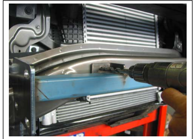
Figure 2: Drill holes to 10mm
