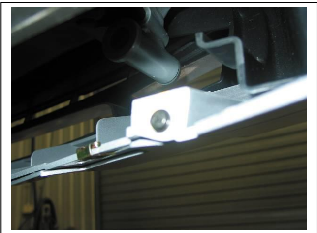
Figure 3 – PK screws on lower rear of bumper.
