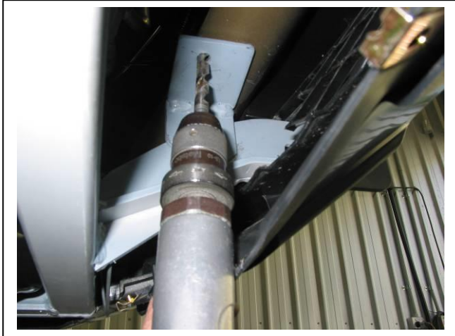
Figure 17 – Shown drilling cross member on passenger side
