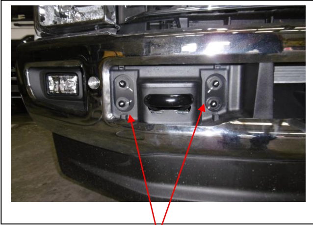
Figure 1: Remove four 18mm head bolts per side.
