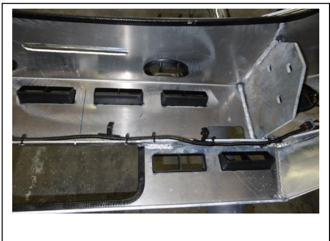
Figure 5: Note wiring on top at winch hole and under on tow point holes
