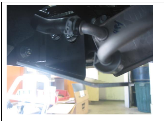
Figure 11: Oil cooler deflector
