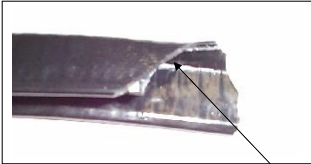
Figure 6 Trim lower edge on an angle.
