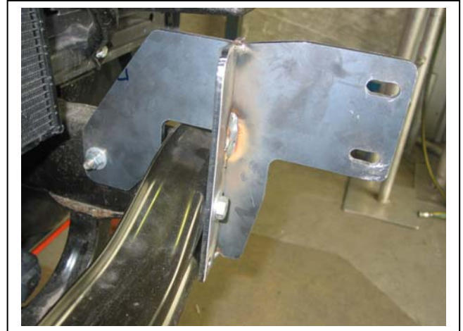
Figure 2: Rear leg fitment to inside of chassis rail.
