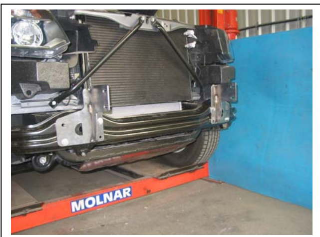
Figure 5: ECB mounts fitted to front of cross member.
