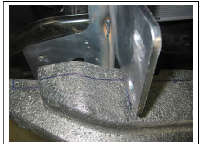
Figure 4: Mark and trim polystyrene infill.
