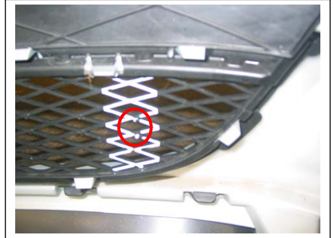
Figure 10: Area to be cut is white. Note: nipples on grille
