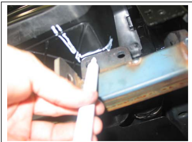
Figure 5: Mark underside of air dam for trim
