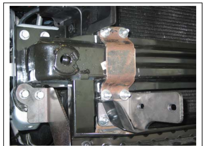
Figure 8: ECB steel saddle fitted
