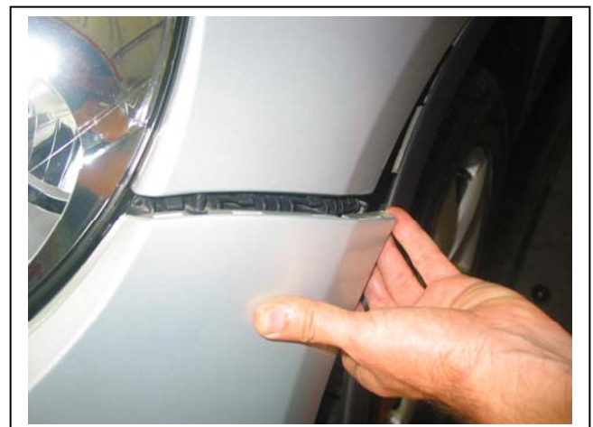
Figure 2: Pull bumper out from guard, then forward
