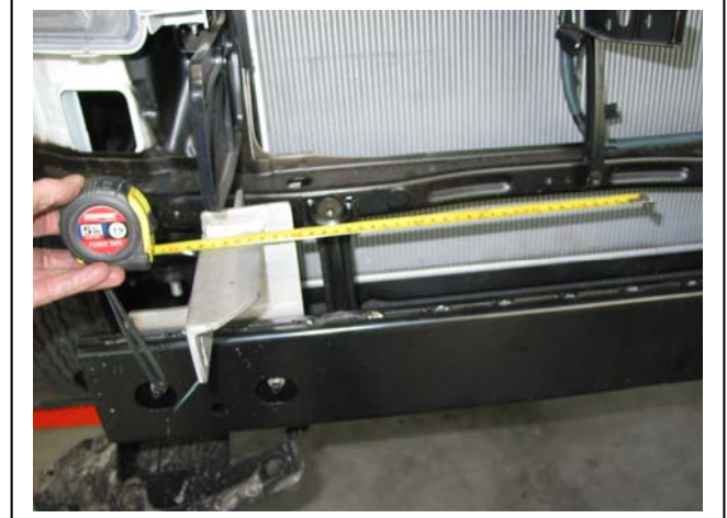
Figure 4 – Drivers side shown centralising steel mounting bracket
