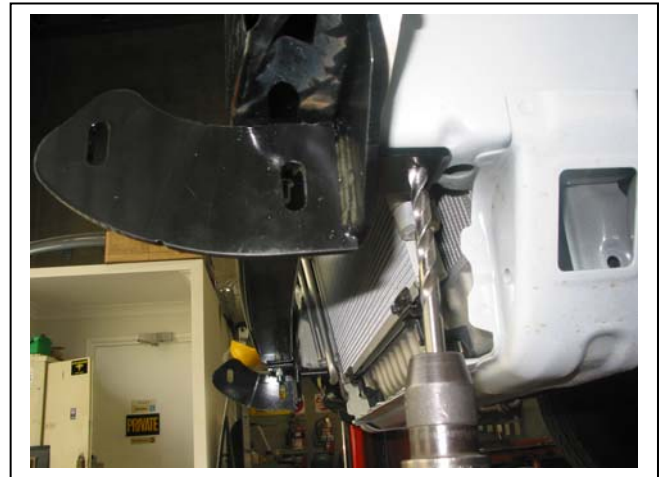
Figure 10 – Shown drilling passenger side chassis
