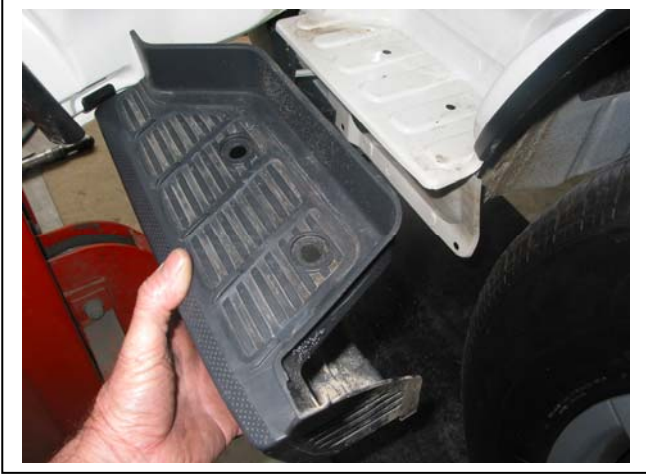
Figure 1 – Shown removing passenger side step infill
