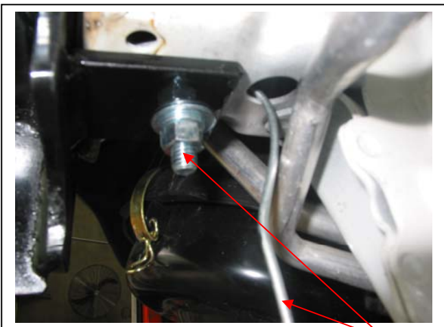
Figure 11 – Driver's side shown 3/8 x 1 1/4 bolt/wire
