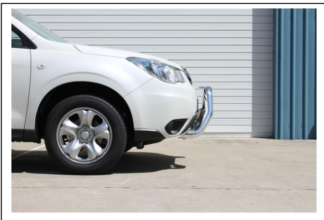
Figure 9: 76mm Nudge Bar side view
