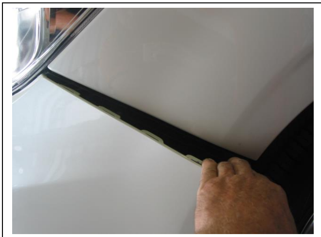
Figure 1: Unclip bumper from guard and light
