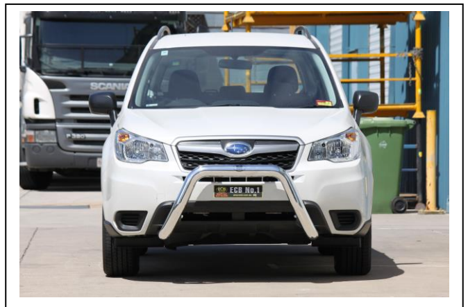
Figure 8: Nudge Bar front view
