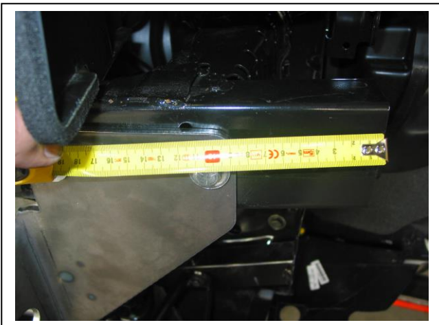
Figure 3: Mark edge of ECB Steel Mounting Bracket on bumper support. (87mm)
