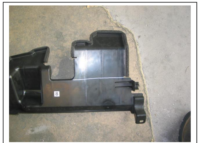
Figure 6: Trim drivers side air ducting.
