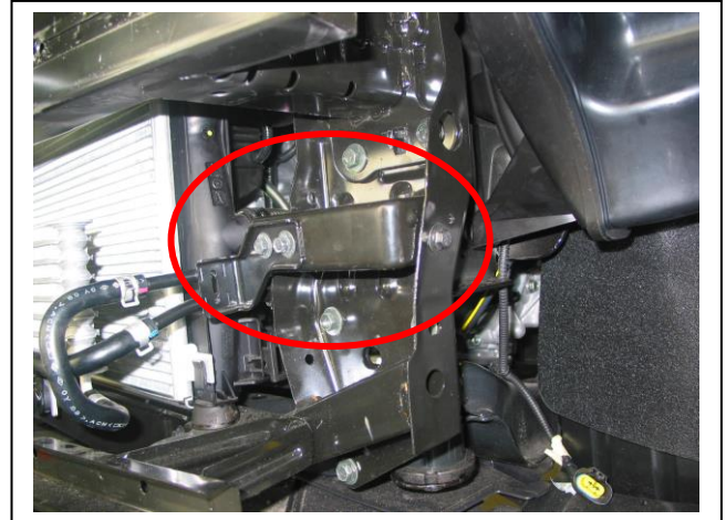
Figure 2: Remove power steering hose mount
