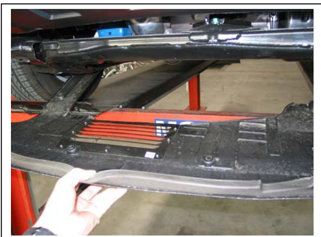
Figure 1 Removing plastic under guard
