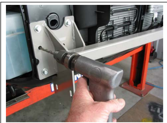
Figure 7 – Shown drilling drivers side – Take extra care not to damage washer bottle with drill bit
