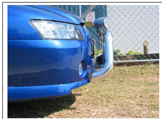
Figure 24 – 76mm Nudge Bar side view shown SV6 shown
