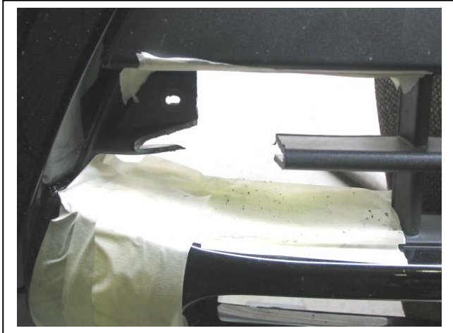
Figure 4: Lower grille trim. Note: Angle of outer cut and trim of bolt area of plastic bumper cover.
