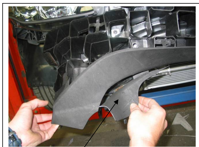
Figure 4: Trim infill on flexible plastic insert to suit ECB steel mounting bracket
