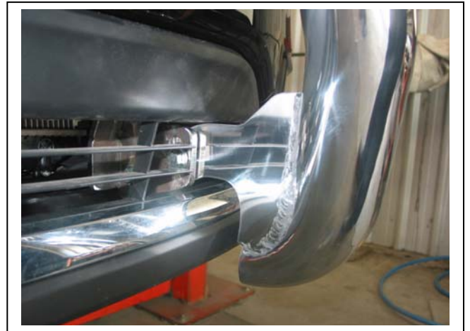
Figure 4: Mounts fitted and bumper refitted to vehicle.
