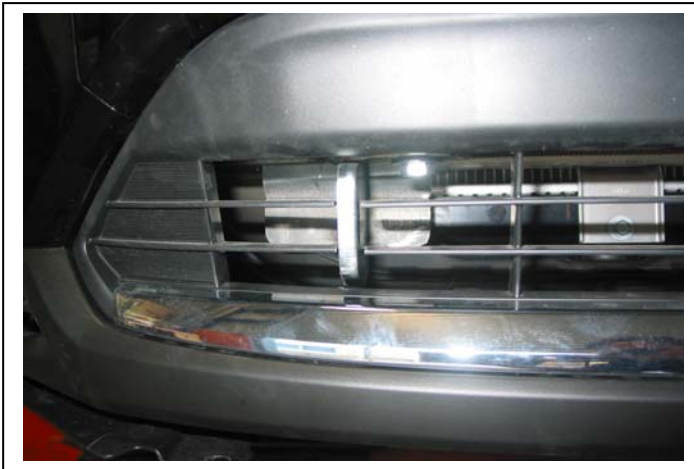
Figure 3: Trim lower grille relative to steel mounts allowing room for Nudge bar to pass thru to outside. Drivers side shown.
