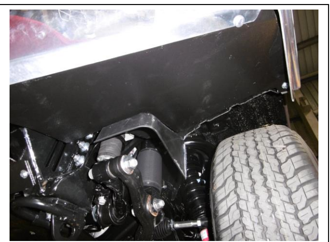
Figure 23: Passenger side guard trimmed.
