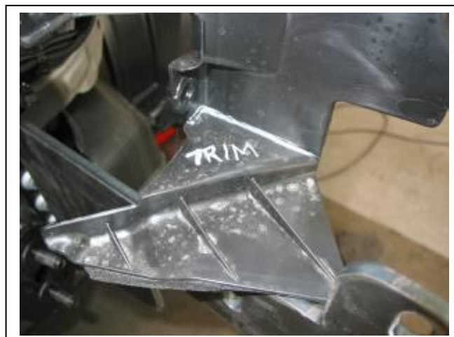
Figure 4: Approximate trim on passengers side shroud.
