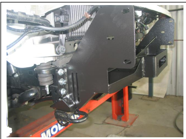
Figure 5: Three bolts to crash can assembly.
