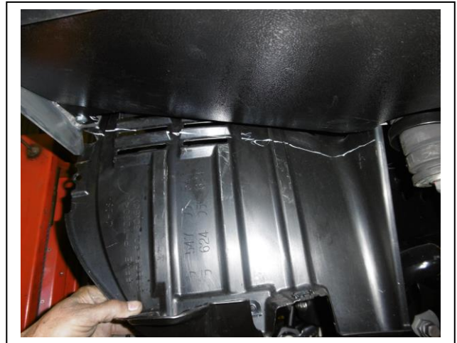
Figure 20: Drivers side guard liner trim line.
