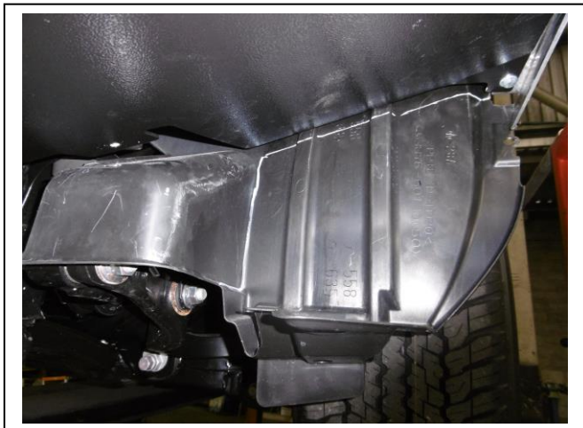
Figure 21: Passenger side guard liner trim line.
