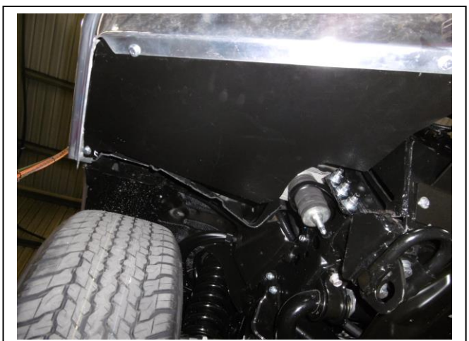
Figure 24: Drivers side guard trimmed.
