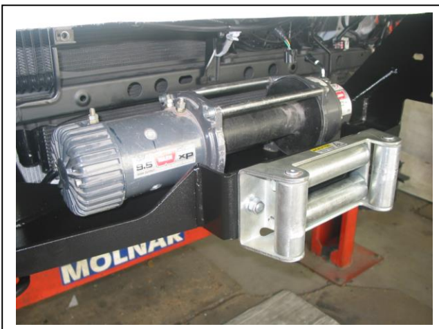
Figure 8: Warn Winch fitted for photo.
