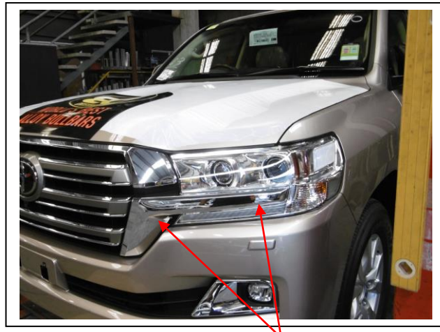
Figure 2: Chrome infill to remove.
