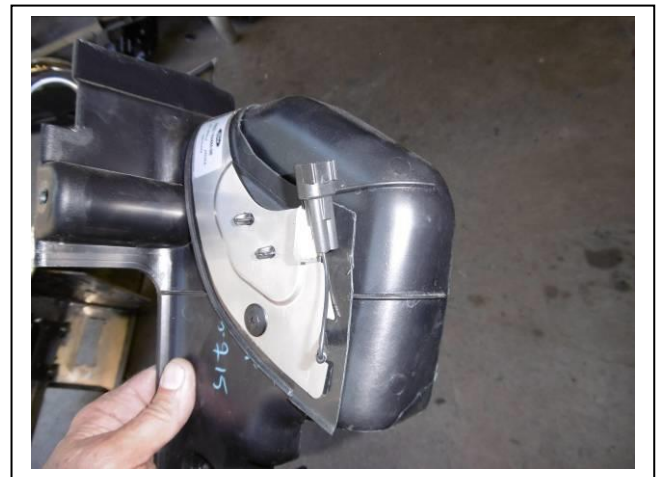
Figure 10: Bend aerial carefully to the shape of the dam and drill in the holes already in place
