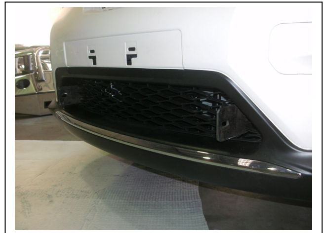
Figure 10: ECB steel mounting bracket with bumper fitted
